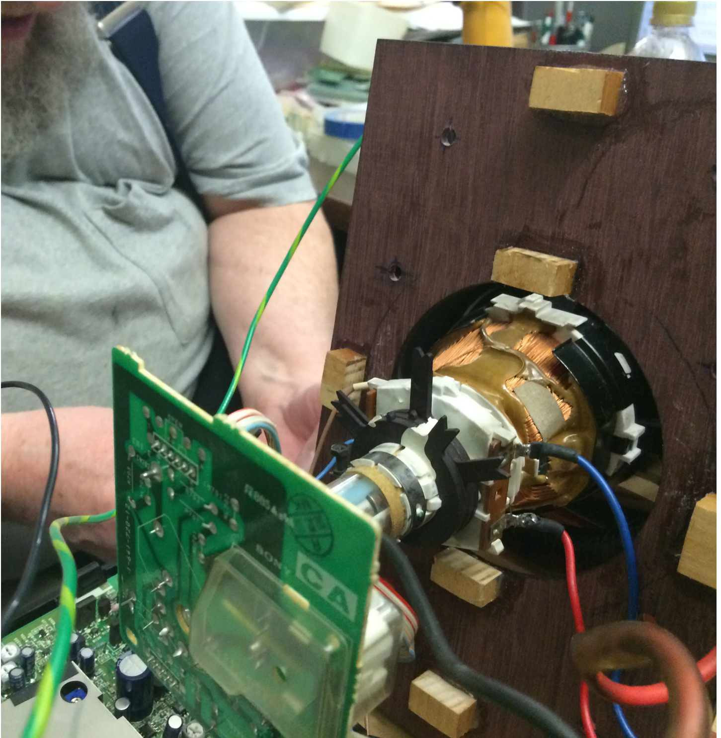
This is the housing for the two vertical yoke system. The wood panel is screwed to the base, and there is a notch in the side to make room for the high voltage wire traveling to the anode cup. The wood blocks help place the coils and angle them properly.
