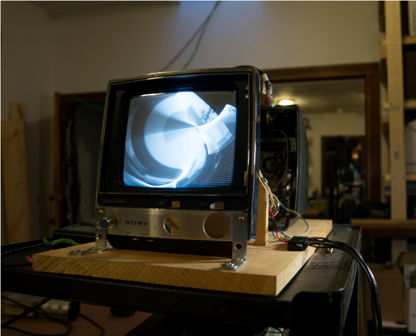
Fully functioning Sony TV-760 Wobulator. S-Coil deflection using 60hz sine wave.
