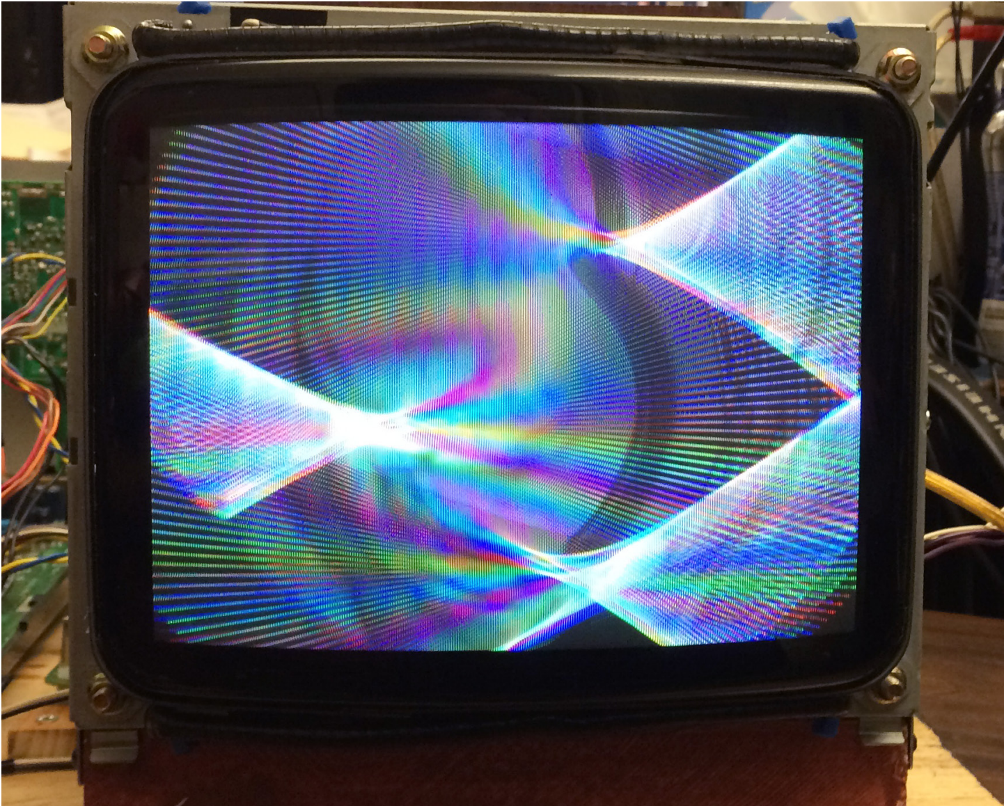
Fully functioning Color Wobbulator. S-Coil deflection using 180hz sine wave.
